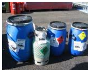
Storage of liquid chemical wastes in chemical-resistant plastic containers
